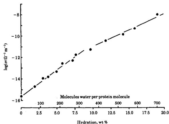
FIG. 3. Variation of the steady-state conductivity  $\sigma$  with hydration for albumin at 294 K.
