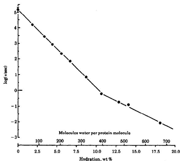
FIG. 2. Variation of the characteristic relaxation time  $\tau$  of the low-frequency dielectric loss peak for albumin as a function of hydration at 294 K.
