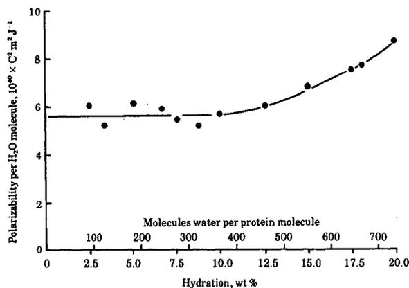
FIG. 4. Variation of the effective polarizability per bound water molecule for albumin as a function of total hydration at 294 K.
