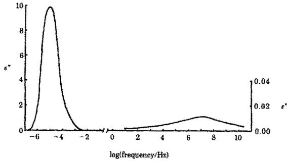
FIG. 1. Frequency variation of the imaginary component of the relative permittivity measured for dry albumin at 294 K.
