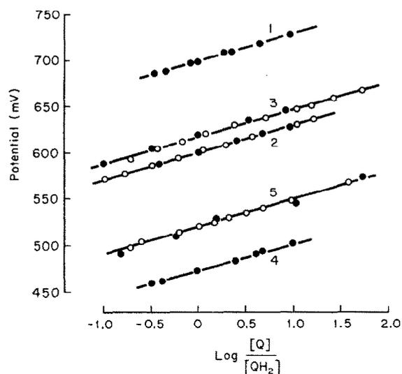
FIG. 1. Electrochemical potential at 25°C in 10% methanol/90% HCl/KCl as a function of the quinone (Q)/hydroquinone (QH<sub>2</sub>) concentration ratio. ●, Quinone/hydroquinone mixtures; ○, quinone/ascorbic acid titrations. Curves: 1, *p*-benzoquinone; 2, methoxyquinone; 3, 2,3-dimethoxyquinone; 4, 2,5-dimethoxyquinone; 5, 2,6-dimethoxyquinone.
